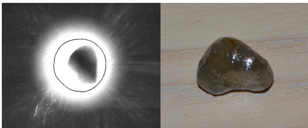
Figure 4 Left: DCT of a rough diamond. Right: Appearance of the rough diamond.
